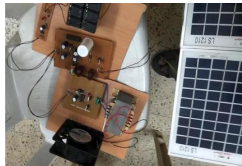
Fig. 6. The kit is connected to solar panel as an input source
