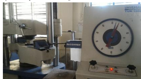
Fig. 6. Test setup for compressive strength in universal testing machine
