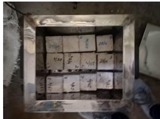
Fig. 5. Specimens under steam curing
