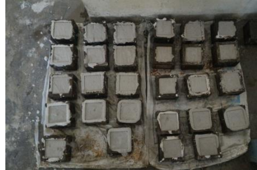
Fig. 4. Lime Pozzolona mortar specimens for different ratios
