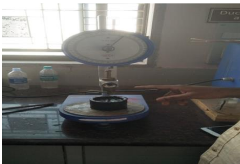
Fig. 5. Test on Penetration Apparatus
