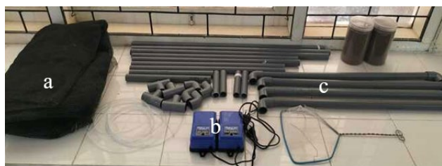
Fig. 1. Fishes rearing (a. Net; b. Water pump; c. PVC pipe)
