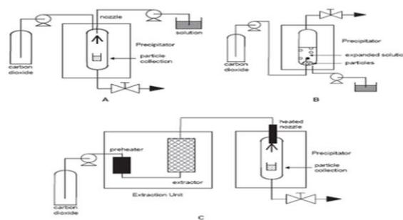
Fig. 5. Schematic diagram of different supercritical fluid spraying
