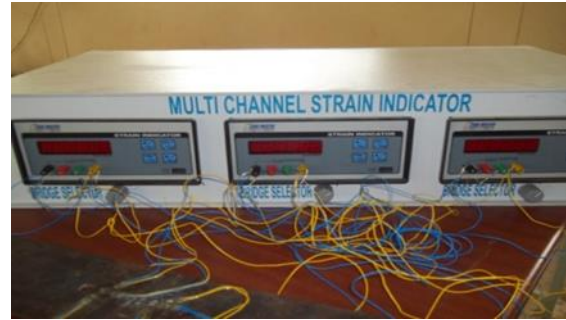
Fig. 5. Strains are measured by multi-channel strain indicator
