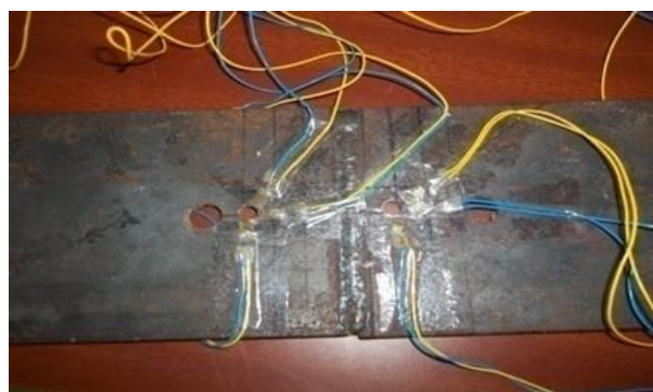
Fig. 4. Strain gauges are bonded to the specimens
