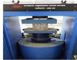
Fig. 3. Split tensile strength test
