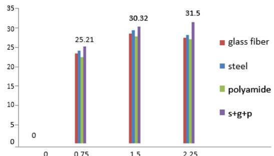
Fig. 8. 7- Day compressive strength of fibres: Percentage of fibres
