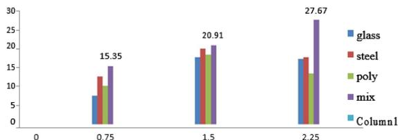
Fig. 6. 28- Day split tensile strength of fibres: Percentage of fibres
