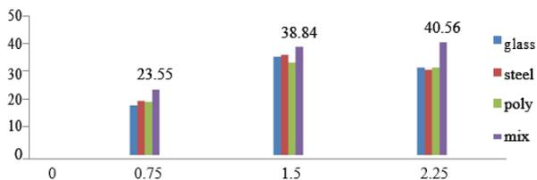
Fig. 7. 7- Day flexural strength of fibres: Percentage of fibres
