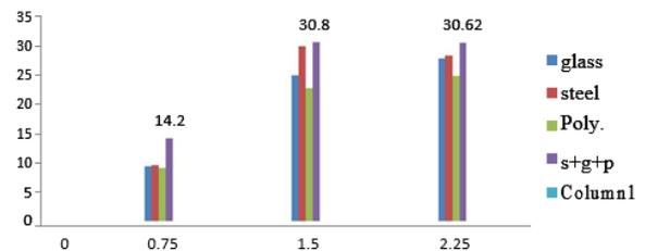
Fig. 9. 28- Day compressive strength of fibres: Percentage of fibres
