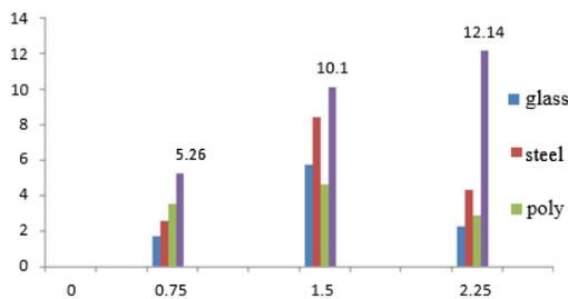
Fig. 5. 7- Day split tensile strength of fibres: Percentage of fibres
