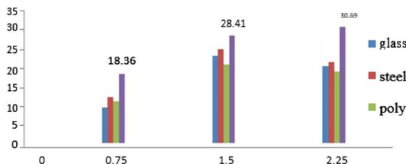
Fig. 8. 28- Day flexural strength of fibres: Percentage of fibres
