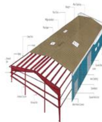
Fig. 2. Components of steel PEB
