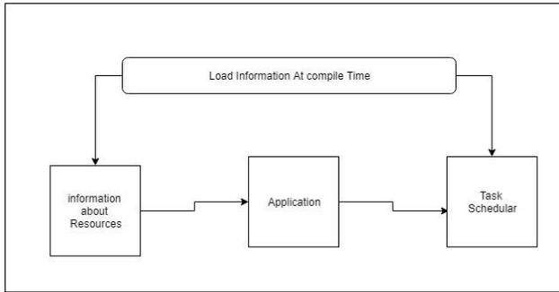
Fig. 2. Working of static load balancing algorithm
