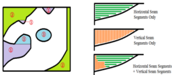
Fig. 6. Left: The target shape S is marked in white. Its complement s can be decomposed into three types of regions: 1) regions that can be reached (seen) from one side of the boundary using horizontal or vertical lines, 2) regions that can be reached from two sides of the boundary and 3) regions that cannot be reached from any side. Right: Removal of a Type-1 region can be accomplished using one kind of seam segments (either horizontal or vertical) while Type-2 region can be removed by carving out a combination of vertical (orange) and horizontal (green) seam segments. Note that Type-3 region cannot be removed by seam segment carving. (Best viewed in color).
