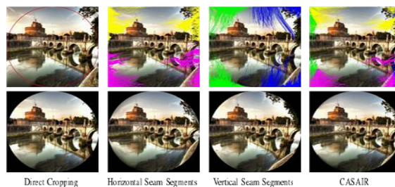
Fig. 7. Content and Shape-Aware Seam Segment Selection First row, from left to right, original image with new boundary highlighted, removing only horizontal seam segments, removing only vertical seam segments, seam segments selected by our method (green, blue, yellow, violet seam segments denote the four type of seam segments, L, R, T, B, respectively). Second row, from left to right, result from direct cropping, result from removing only horizontal and vertical seam segments, result produced by our method.
