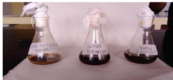
Fig. 1. 2.5ml of silver nanoparticles extract resulted in change in color augmented with silver nitrate after one hour of incubation at temperature 60 0 C and 100 0 C
