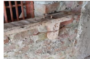
Fig. 3. Permanent instrument for making stirrups and ties
