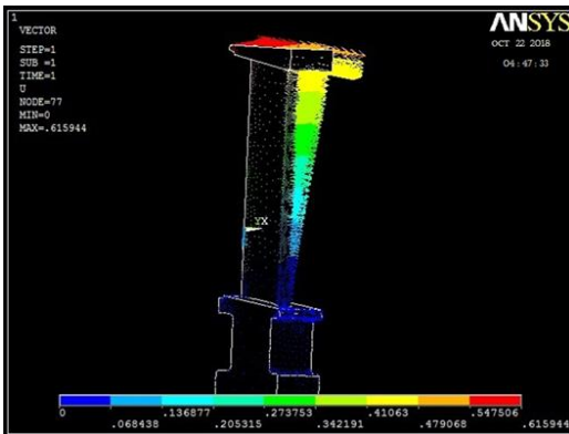
Fig. 14. HP blade vector mode analysis
