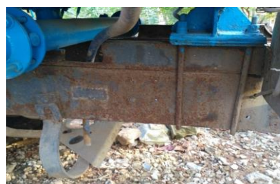
Fig. 5. Corrosion on vehicle chassis
