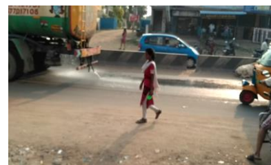
Fig. 7. Water leaks on road from tanker lorry
