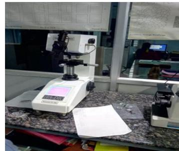
Fig. 4. Vickers micro hardness tester
