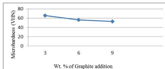
Fig. 5. Graph showing wt. % of Graphite vs. Micro-Hardness
