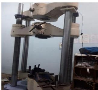
Fig. 2. Universal Testing Machine
