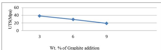
Fig. 3. Graph showing wt. % of graphite vs. UTS
