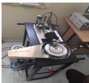
Fig. 6. Pin-on-disc apparatus
