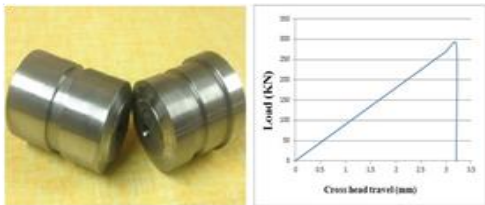
Fig. 4. Curve for groove size: \phi 24.0 mm
