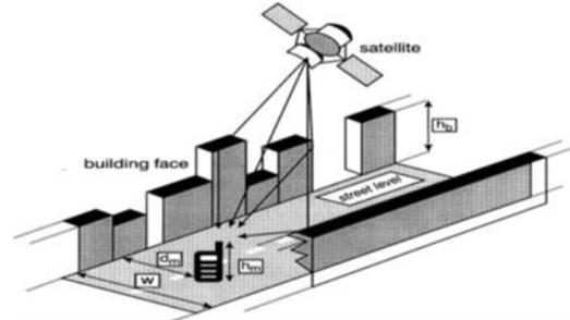
Fig. 5. Path Geometry for mobile satellite
