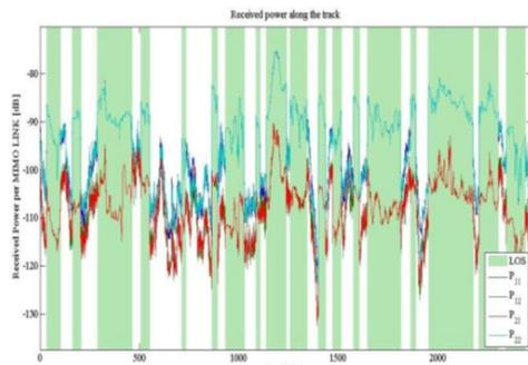
Fig. 9. Simulated Time series of LMS Channel using geometry based stochastic methods
