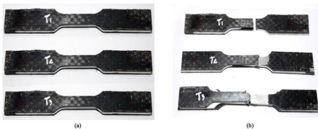
Fig. 2. The specimen (a) Before tensile test, (b) After the fracture
