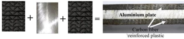
Fig. 1. Schematic illustration of aluminium sandwich carbon fibre reinforced composites
