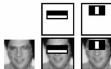
Fig. 2. Finding the eyes using Haar-features
