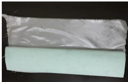
Fig. 10. Image showing glass fibre and wing section before layup and application of resin.
