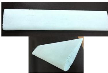
Fig. 9. Image showing foam core wing and cross section of the wing with NACA 0015 aerofoil
