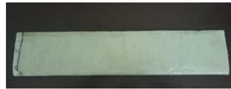
Fig. 11. Prototype model of wing with foam as core and skin as composite woven material
