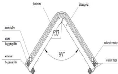
Fig. 3. Vacuum system for curved-beam element
