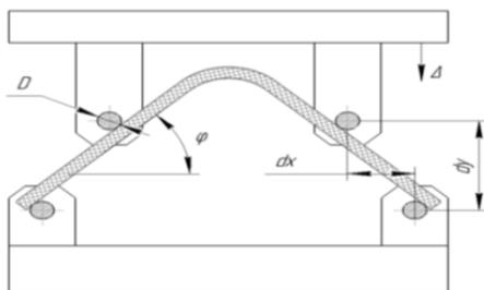
Fig. 4. Testing scheme for curved-beam element
