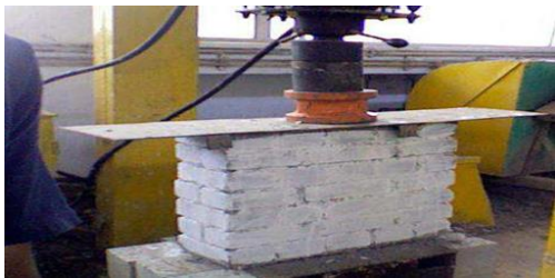
Fig. 1. Prism test on fly ash bricks
