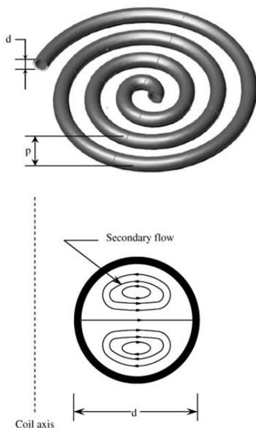
Fig. 3. Spiral capillary tube
