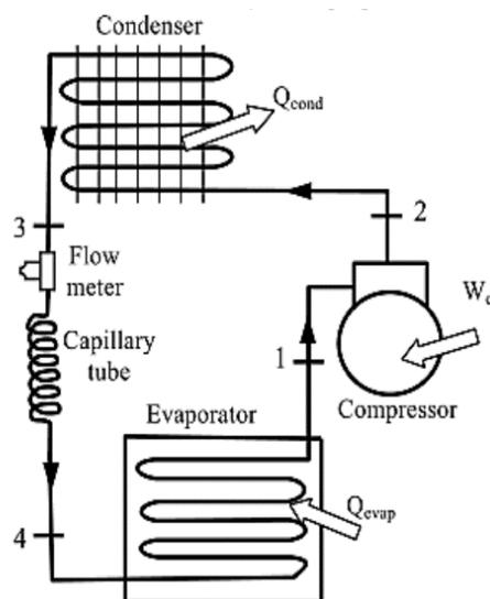
Fig. 1. Block diagram of VCRS cycle
