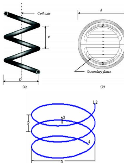
Fig. 4. Helical capillary tube
