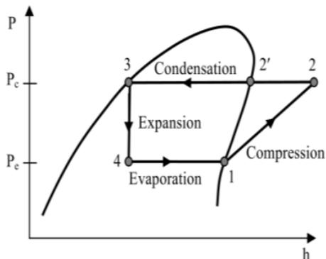
Fig. 2. P-h diagram of VCRS cycle
