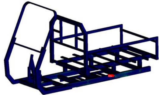
Fig. 11. Maximum equivalent stress was found to be below 240 MPa
