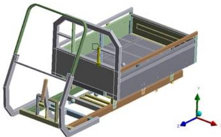
Fig. 8. Load of 1200 N applied on the front driver seat area
