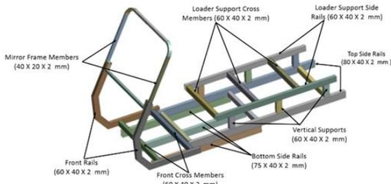
Fig. 2. Initial reverse engineered design of vehicle chassis
