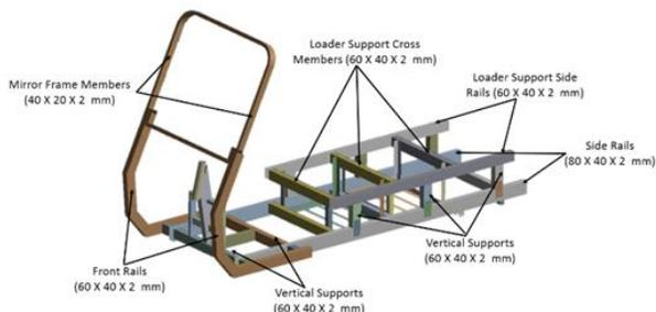
Fig. 3. Modified reverse engineered design of vehicle chassis
