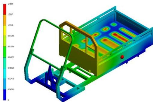
Fig. 13. Maximum deflection on loader frame was found to be 1.45 mm
