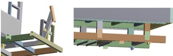
Fig. 9. Front suspension and rear leaf spring eyes surface are assigned as fixed support in all the directions
