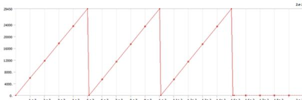
Fig. 10. Bump Profile applied on loader vehicle
