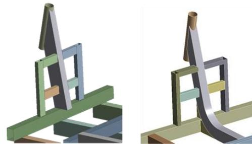
Fig. 4. Front suspension of existing vehicle and modified Front suspension of modified vehicle
