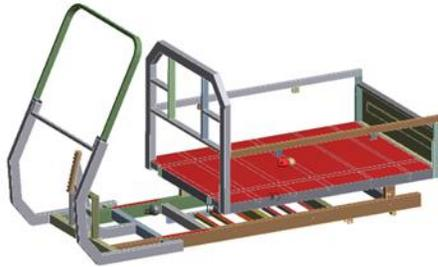
Fig. 7. Load of 10,000 N (1 tonne) applied on the carrier
