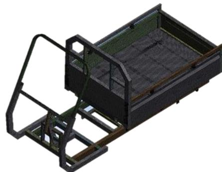
Fig. 6. FE model of the modified chassis
