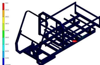
Fig. 15. Maximum equivalent stress on chassis structure is found to be 225.12 MPa
