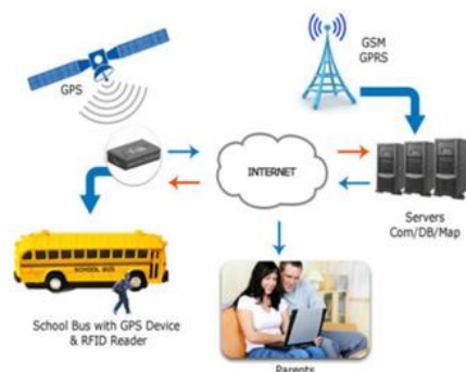
Fig. 4. Block diagram of GNSS based monitoring system
