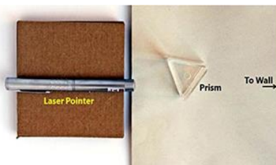
Fig. 9. Diagram of setup for measuring the index of refraction of a liquid using a laser pointer and a hollow triangular prism (not to scale; based on the diagram in Nierer, 2002)
