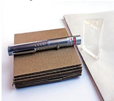
Fig. 10. Adjust the height of the laser pointer with pieces of cardboard. The beam of the laser should hit the prism about halfway up the prism's side
