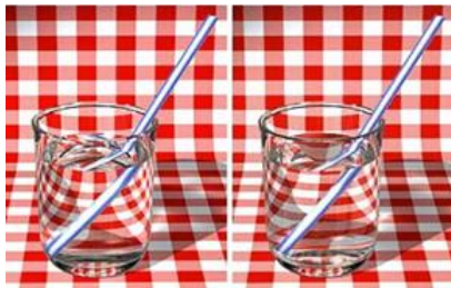
Fig. 1. These two figures demonstrate refraction by liquids. One tumbler contains plain water, and the other contains sugar-water. Which glass has which liquid? (Wood, 2003) (Images © Robin Wood, 2003, used with permission.)
