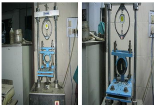
Fig. 2. Photographic views of the fabricated Interlayer Bond Strength device
