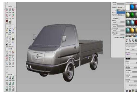
Fig. 3. Design and Digital Prototype of a Light Commercial Vehicle using ALIAS
