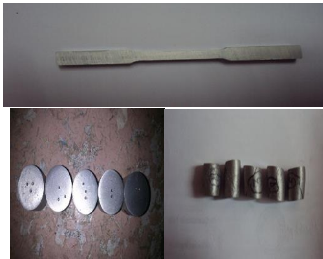
Fig. 4. Test specimen for tensile, hardness and compressive test
