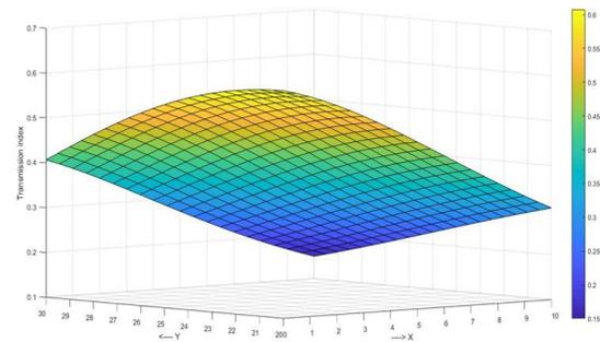
Fig. 8. Transmission index of 8 UPS parallel Manipulator for  $R_b=60, R_p=30$  &  $z=28$ , Twist angle  $\Psi=90^\circ$ , Tilt angles  $\theta=70^\circ, \dot{\theta}=90^\circ$
