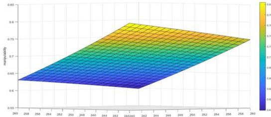
Fig. 5. Manipulability index of 8 UPS parallel Manipulator for  $R_b=30, R_p=20$  &  $z=28$ , Twist angle  $\Psi=90^\circ$ , Tilt angles  $\theta=70^\circ, \dot{\theta}=90^\circ$
