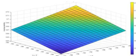
Fig. 3. Manipulability index of 8 UPS parallel Manipulator (for  $R_b=60, R_p=30$  &  $z=20$ , Twist angle  $\Psi=10^\circ$ , Tilt angles  $\theta=10^\circ, \phi=10^\circ$ )
