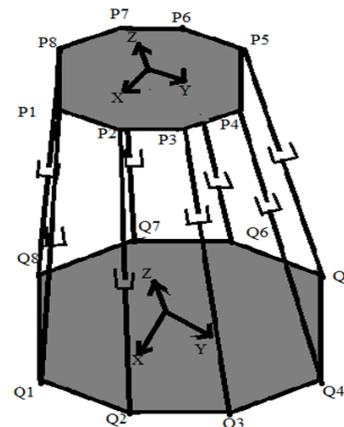
Fig. 1. Kinematic model of 8-UPS parallel manipulator
