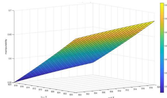
Fig. 4. Manipulability index of 8 UPS parallel manipulator for  $R_b=70, R_p=30$  &  $z=35$ , Twist angle  $\Psi=8^\circ$ , Tilt angles  $\theta=9^\circ, \phi=9^\circ$
