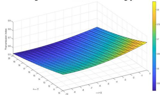
Fig. 7. Transmission index of 8 UPS parallel Manipulator for  $R_b=30, R_p=20$  &  $z=35$ , Twist angle  $\Psi=80^\circ$ , Tilt angles  $\theta=90^\circ, \dot{\theta}=90^\circ$
