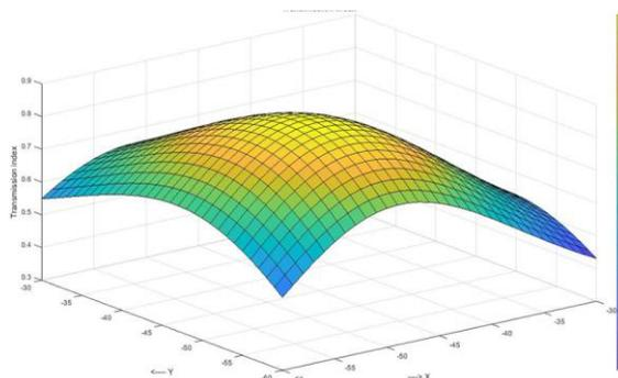
Fig. 6. Transmission index of 8 UPS parallel Manipulator for  $R_b=70, R_p=30$  &  $z=20$ , Twist angle  $\Psi=100^\circ$ , Tilt angles  $\theta=100^\circ, \dot{\theta}=100^\circ$
