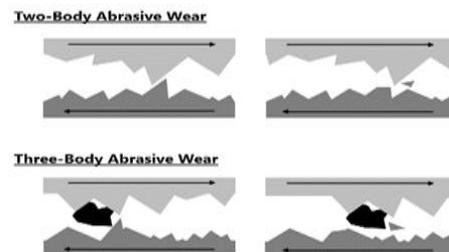
Fig. 1. Abrasive wear
