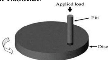
Fig. 3. Schematic diagram of pin on disc machine
