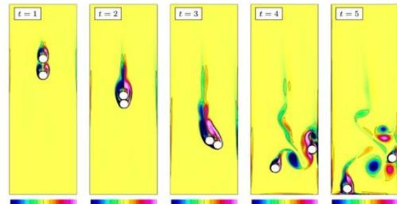
Fig. 8. Vorticity contours in different time step. Scale (-3.6, 3.6) [2]
