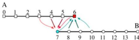
Fig. 2. Overlapping of two 1D meshes. Interpolation of fringe points [6]
