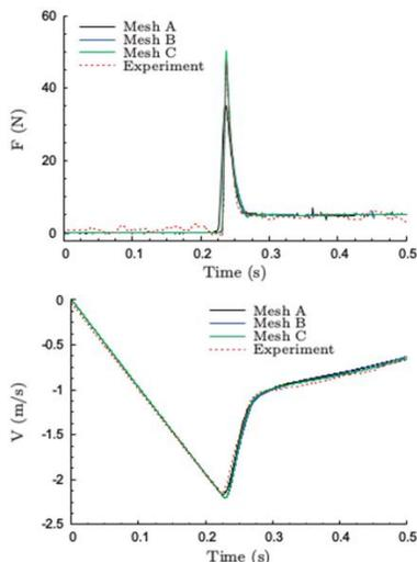
Fig. 7. Temporal Plots of Force and velocity for free falling wedge [6]
