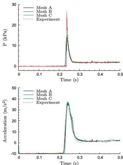
Fig. 6. Temporal Plots of Pressure and acceleration for free falling wedge [6].
