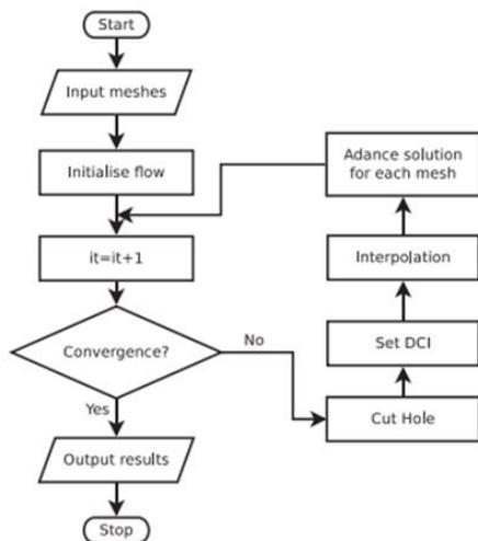
Fig. 4. Flow chart of overset grid simulation [6].
