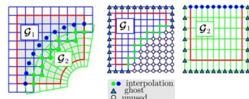
Fig. 1. Interpolation on overset grid [2].
