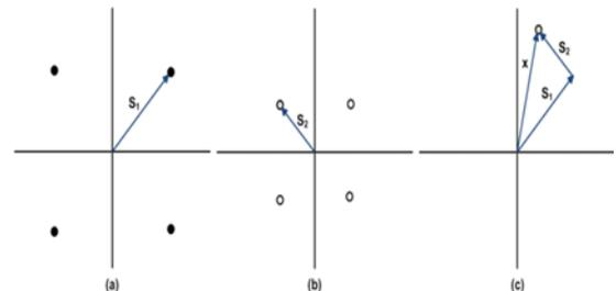
Fig. 3. An example of SC encoding (a) signal constellation of user 1 (b) signal constellation of user 2 (c) constellation of superposed signal.
