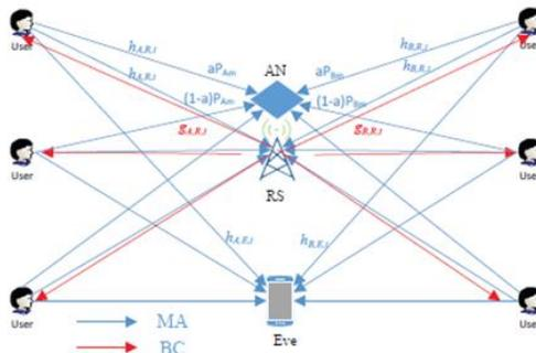
Fig. 1. System model of the security transmission in two-way relay wireless network
