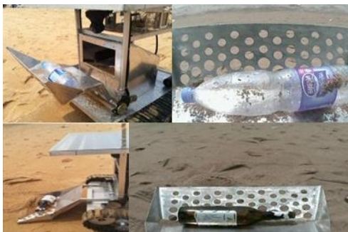
Fig. 8. The garbage collection test (The large garbage)
