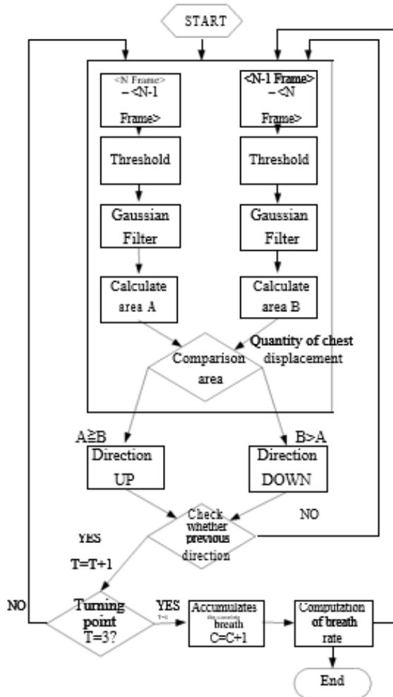
Fig. 5. Flowchart of breath rate detection
