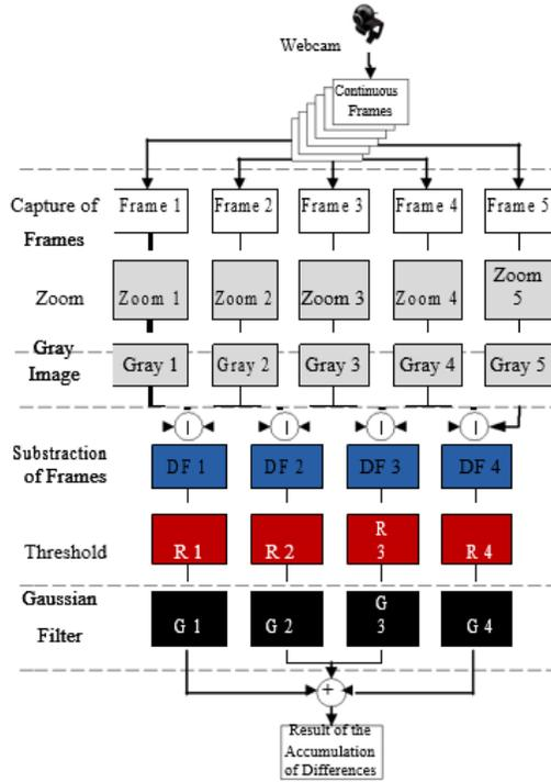
Fig. 2. Flowchart of the accumulation of the differences and the elimination of noise
