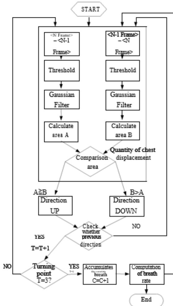
Fig. 5. Flowchart of breath rate detection
