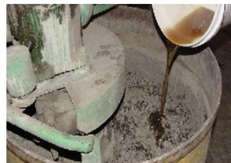
Fig. 2. Alkaline solution mix in preparation of geopolymer concrete
