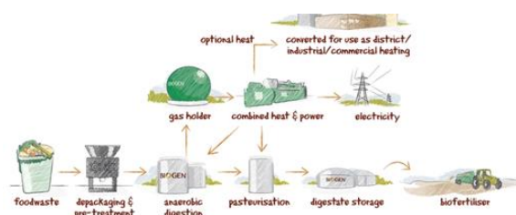
Fig. 2. Anaerobic digestion process
