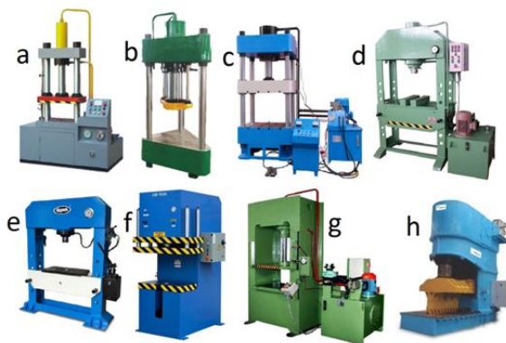
Fig. 1. Various types of hydraulic press frames. (a) Two Column Press, (b) Three Column Press (c) Four Column Press (d) Fabricated Four Column Press (e) Fabricated Two Column Press or H-Frame Press (f) C-Frame Press (g) Close-Frame Press (h) Fabricated Chamber Press
