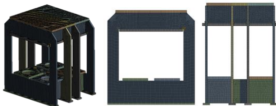
Fig. 3. Element model with 2D shell elements
