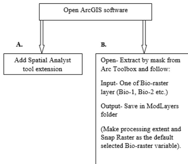
2) Converting environmental raster to ASCII format
