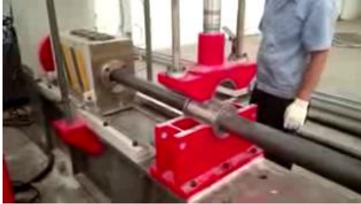
Fig. 4. Actual assembly of automatic clamping fixture
