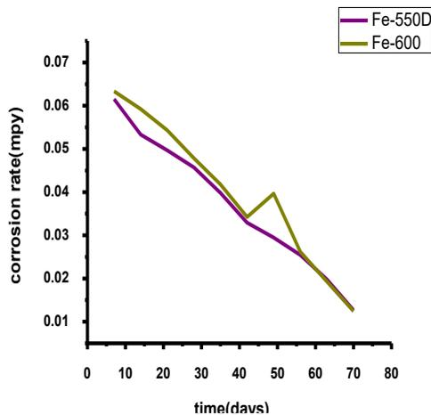
Fig. 4. Variation of corrosion rate (mpy) with exposure time of TMT steels in fresh water
