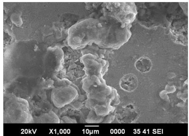
The surface morphology obtained from scanning electron microscope (shown in Fig. 7 and 8) indicated that both of these reinforcing steel bars suffered from pitting corrosion, since the formation of pits were seen very clearly from surface analysis.
