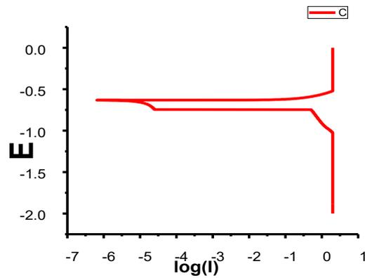
Fig. 5. Tafel polarization curve of TMT Fe 600 EQR steel in 3.5% NaCl
