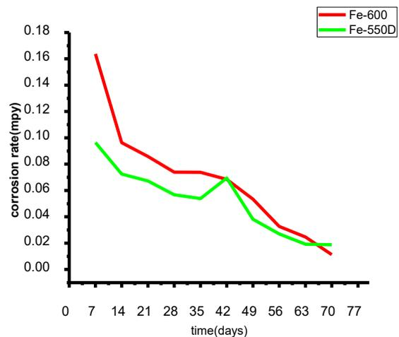
Fig. 3. Variation of corrosion rate (mpy) with exposure time (days) of TMT steels in 3.5%NaCl
