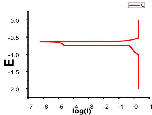
Fig. 5. Tafel polarization curve of TMT Fe 600 EQR steel in 3.5% NaCl
