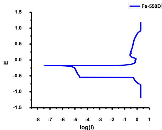
Fig. 6. Tafel polarization curve of TMT Fe 550D steel in 3.5% NaCl
