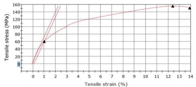
Fig. 9. Tensile stress vs Tensile Strain of 0.3wt % MWCNTs/GNPs
