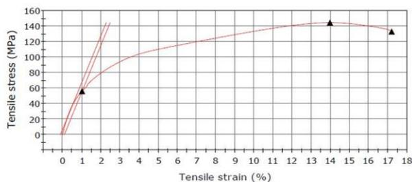
Fig. 5. Tensile stress vs Tensile Strain of 0.2wt % GNPs
