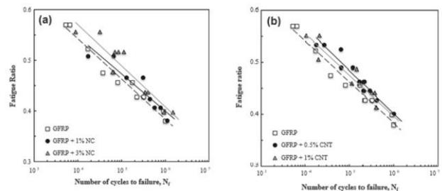
Fig. 14. Fatigue ratio against the number of cycles to failure under tension-tension loading: (a) Nano clay filled GFRP and (b) Carbon nanotube enhanced composite
