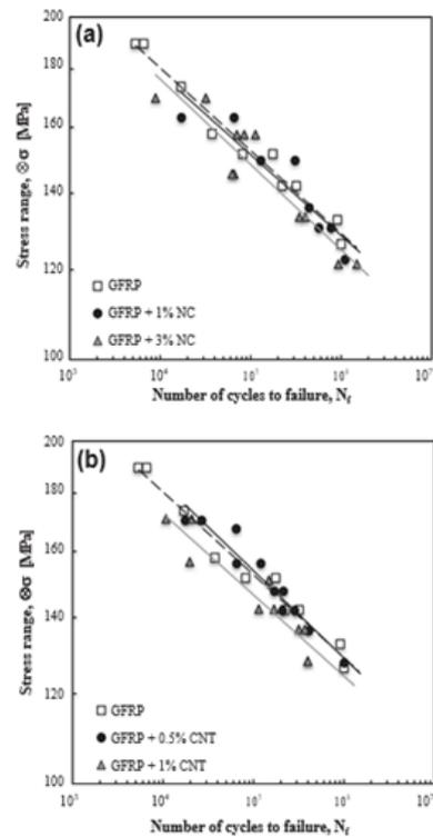
Fig. 13. Effect of nanoparticle addition on GFRP composites under tension-tension fatigue loading: (a) Nano particles and (b) Carbon nanotubes
