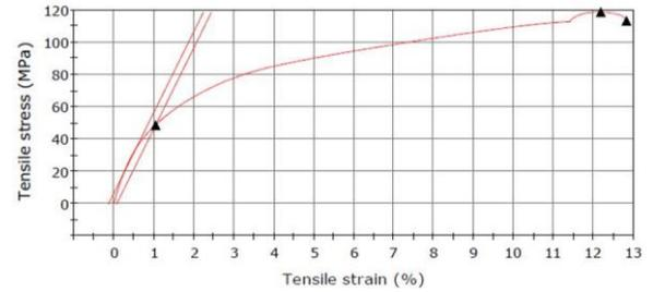
Fig. 6. Tensile stress vs Tensile Strain of 0.3wt % GNPs
