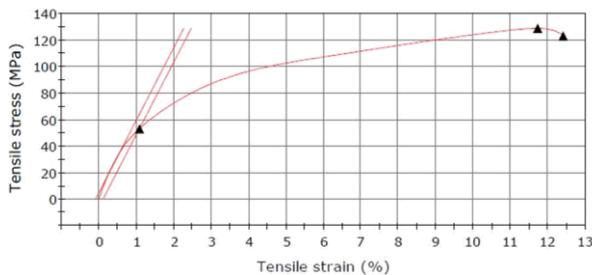
Fig. 4. Tensile stress vs Tensile Strain of 0.1wt% GNPs
