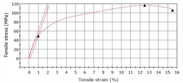
Fig. 8. Tensile stress vs Tensile Strain of 0.2wt % MWCNTs/GNPs
