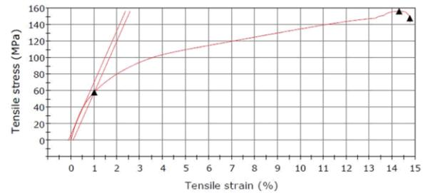
Fig. 7. Tensile stress vs Tensile Strain of 0.1wt % MWCNTs/GNPs
