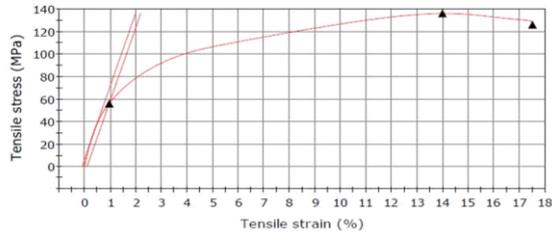
Fig. 1. Tensile stress vs Tensile Strain of 0.1 wt % MWCNTs
