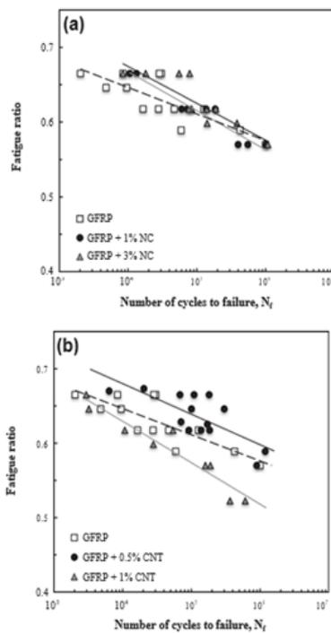
Fig. 12. Fatigue ratio against the number of cycles to failure under 3 PB loading: (a) Nano clay filled GFRP (b) Carbon nano tube enhanced composite
