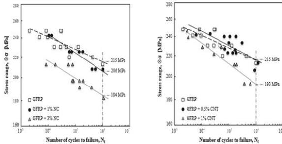
Fig. 11. Effect of nano clay and carbon nano tubes addition on GFRP composites under three point bending fatigue loading
