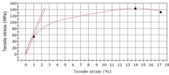
Fig. 3. Tensile stress vs Tensile Strain of 0.3wt % MWCNTs
