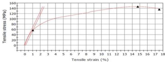
Fig. 2. Tensile stress vs Tensile Strain of 0.2 wt % MWCNTs
