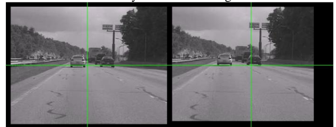
Fig. 3. (a) Unstable input frame (b) Stable output frame for "Shaky Car" video frame using block matching estimation.
