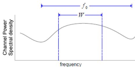
Fig. 4. Typical flat fading channel
