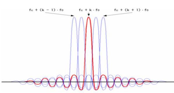
Fig. 1. OFDM - number of closely-spaced orthogonal sub-carriers
