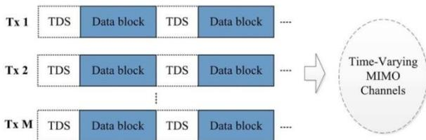
Fig. 5. Frame structure of MIMO TDS-OFDM.
