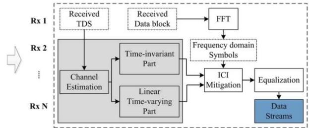
Fig. 6. Receiver side of MIMO TDS-OFDM with ICI mitigation.
