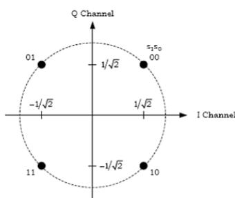
Fig. 2. QPSK Constellation Mapping
