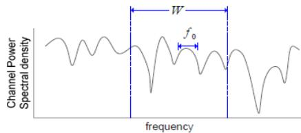
Fig.3. Typical frequency-selective fading channel
