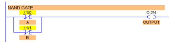
[7] Fig. 3. Ladder logic of NAND Gate
