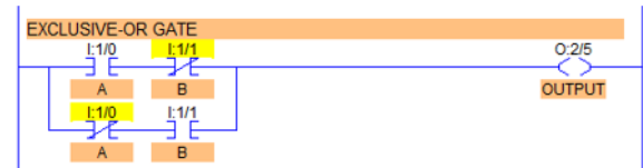
[7] Fig. 4. Ladder logic of Exclusive-OR Gate
