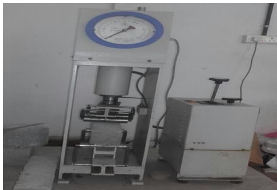
Fig. 8. Specimen loaded to failure in flexural strength testing machine
