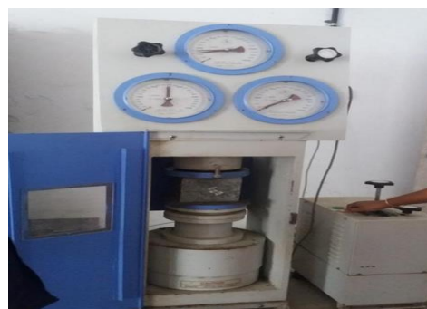
Fig. 7. Specimen loaded to failure in compression
