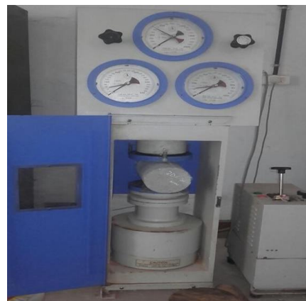
Fig. 11. Specimen loaded to failure in tensile strength test
