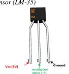
The LM-35 sensor or temperature sensor is used to detect the temperature. It returns the analog value which is then converted to digital form with the help of formula.
