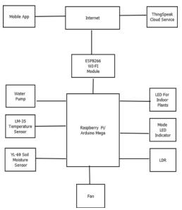
In automatic mode, the user will be asked to provide a threshold value for the data being collected. If the value goes beyond the threshold value, the appropriate function would be performed. Moreover, the data obtained from the sensors could be used to analyse the cost of water and electricity. This would help farmers to analyse the profits and the investment. We can also use the data from weather forecasting services for more efficient use of water.
