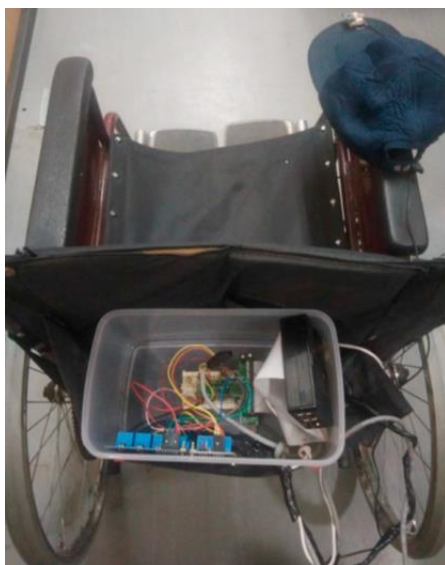
Fig. 9. Head motion controlled wheelchair
