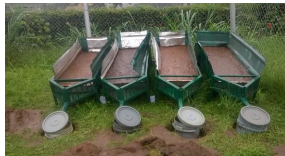
Fig. 1. Setup of the erosion rigs for the erosion investigation
