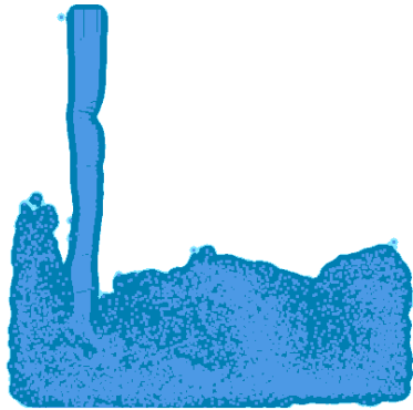
Fig. 2. Grid based 2D simulation of filling water in a glass
